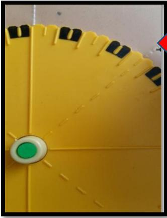
3. Count around using tactile ridges in 5° intervals to mark on film required angle.
